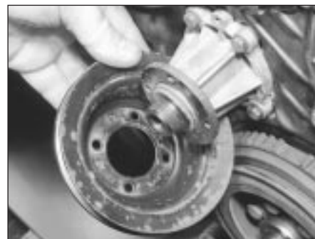
5.29 Removing the water pump pulley (M40 engine)
