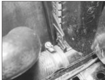
4.3b Bottom hose connection to the radiator
