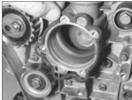
7.24 New outer gasket on the M40 engine water pump
