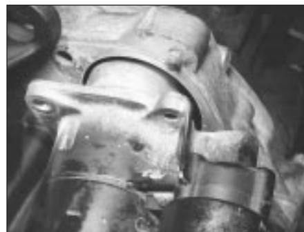
20.4b Withdrawing the starter motor from the M40 engine
