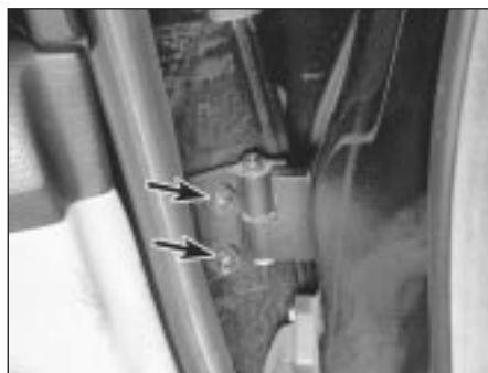
13.5 Remove the nuts (arrowed) and detach the door from the hinges
