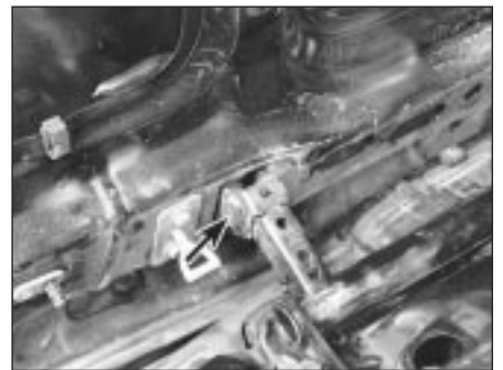
10.12 Unscrew the hinge through-bolts (arrowed)
