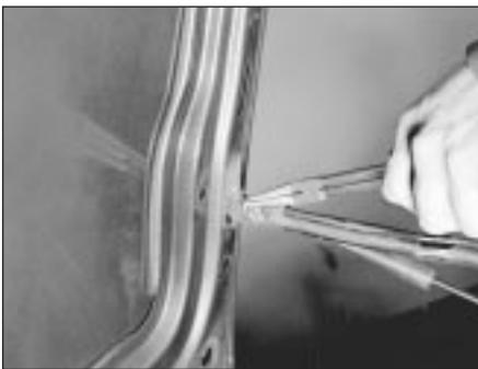
10.9 Pull off the clip with needle-nose pliers
