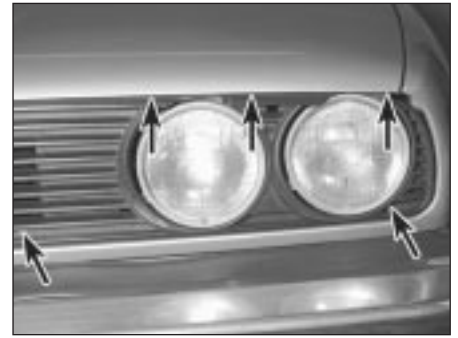
9.2b Side grille screw locations (arrowed)
