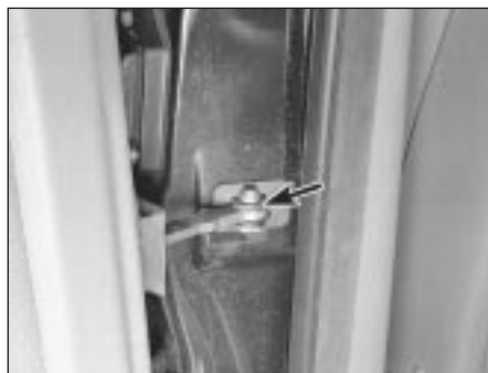
13.4 Detach the circlip (arrowed) from the tapered end of the pin
