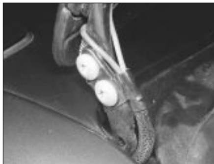
14.9 Tailgate window mounting screws (5-Series)
