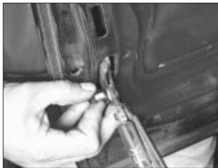
10.10 Support the bonnet and withdraw the pin
