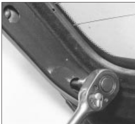
14.14 Unscrewing the hinge mounting bolts (5-Series)
