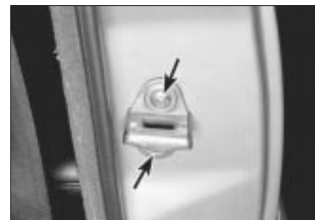
13.7 The door lock striker position can be adjusted after loosening the screws (arrowed)
